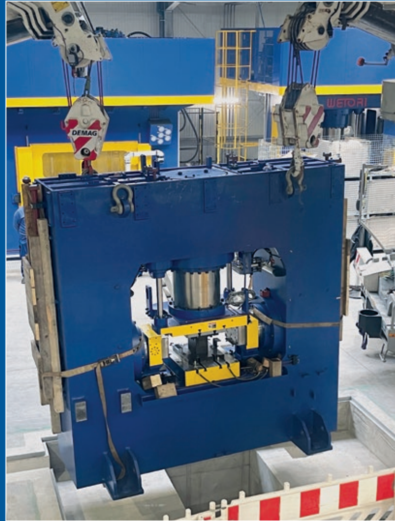
Construction of another hydroforming press (hydroforming) - Pressing force 1200 tons in March 2023.
